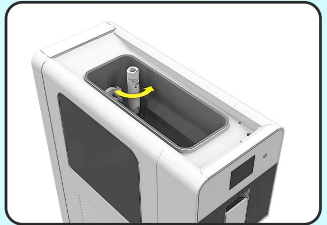
4 Pour the mixture into the upper tank and wait for the cylinder to fill up. This will occur when no more air bubbles exit the hole in the mixing pipe.
